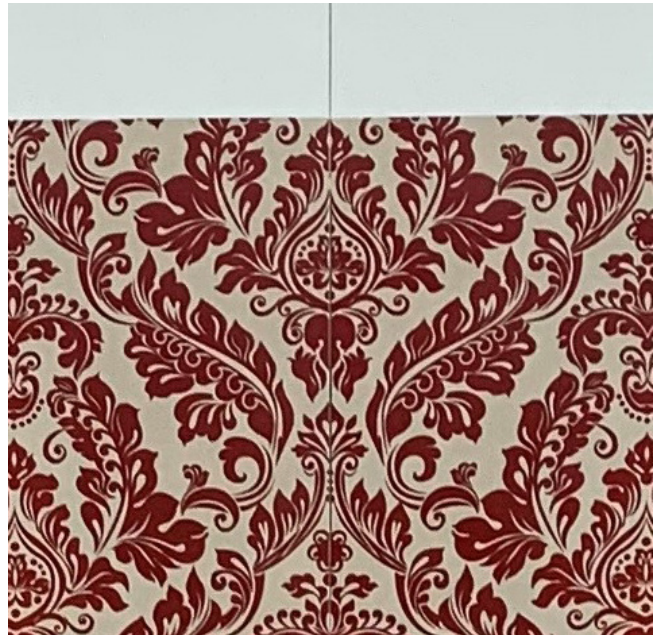
High resolution images showing dimensional and color consistency of wallpaper panels from beginning of the roll – panel 1 (left side) to end of roll – panel 13 (right)
